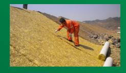
The iGGmat product group includes stitched erosion control and fiber mats. iGGmat erosion control mats are predominantly made of natural fibers, such as coir, straw or a mixture of these. The fibers are sewn in the desired mixture ratio with two carriers made of PP netting or lightweight jute fabric using quilting fibers made of PP or jute.
